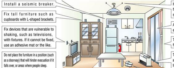
Hanging lights are prevented from falling by suppressing shaking with wires and chains.
